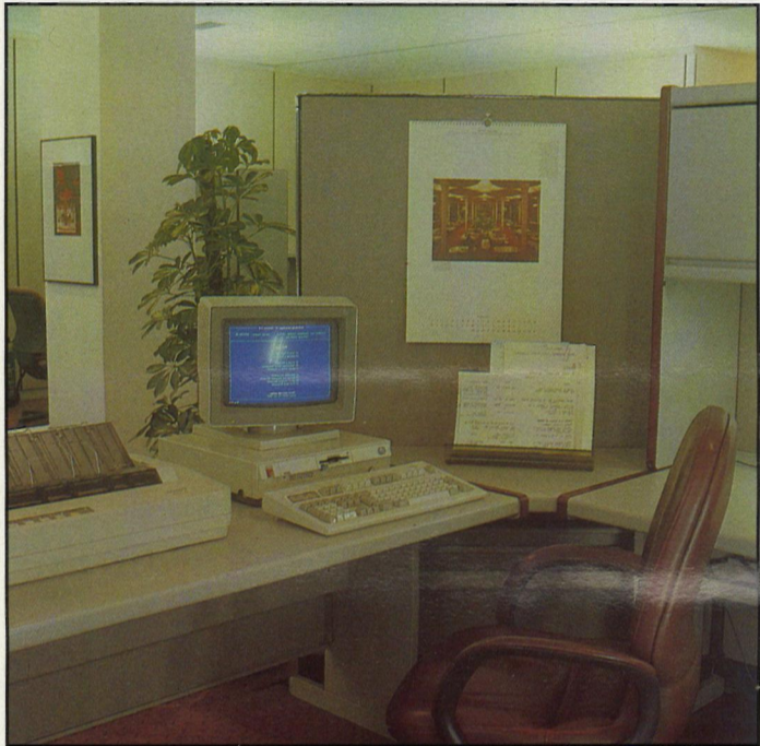
Conventional overhead lighting, showing reflections in visual displays.
